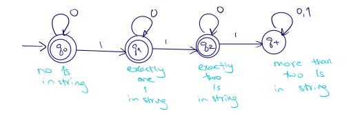
A state diagram for a finite automaton that recognizes  $\{w \mid w \text{ contains more than two 1's}\}$  is
