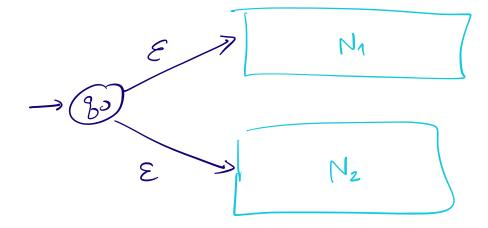
Formal construction: Let  $N_1 = (Q_1, \Sigma, \delta_1, q_1, F_1)$  and  $N_2 = (Q_2, \Sigma, \delta_2, q_2, F_2)$  and assume  $Q_1 \cap Q_2 = \emptyset$ and that  $q_0 \notin Q_1 \cup Q_2$ . Construct  $N = (Q, \Sigma, \delta, q_0, F_1 \cup F_2)$  where
